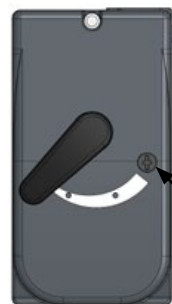
Diversion to the heating circuit. Priority position.
